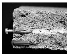
Plug anchor - NO extrusion & NO bonding
