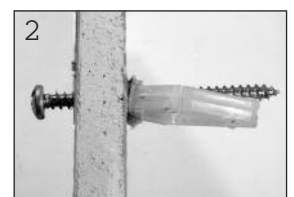
Screw at angle in competitive anchor—misses apex; NO holding power
